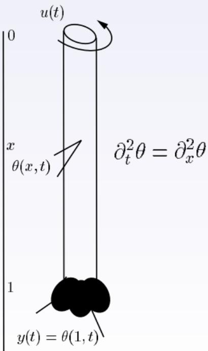
FIG. 15: Vibrations de torsion.
